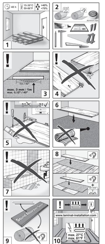
**Preparation:** Please store the packets 48 hours prior to installation under the same climatic conditions (temperature and moisture) as the actual installation process [1]. Important pre-condition for proper fitting and long-term durability of the laminated flooring is a room temperature of  $15 - 30^{\circ}$ C /  $59 - 86^{\circ}$ F and a relative humidity of around 40 - 70%.
